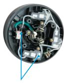
GDT / TMOV hybrid circuit eliminates leakage and follow on current extending the life of the surge protector.
