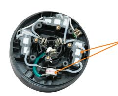
Gas Discharge Tube / MOV Circuit designed to eliminate leakage and follow on current extending the life of the surge protector.
